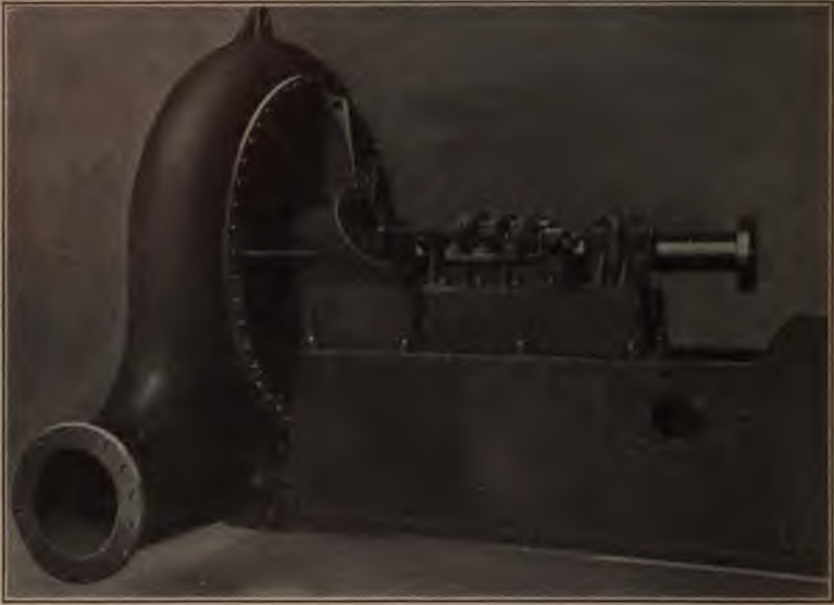
Centrifugal Pump of Hydraulic Dredge. Figure 105.
